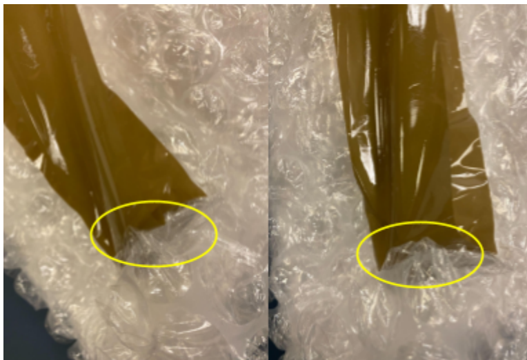
Fig 11: Removing the adhesive packing tape physically pulls on the delicate surface of the bubble wrap, causing mechanical damage. Risks a shorter reuse of the material.
